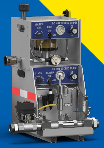
Optional add-on fluid injection system delivers a mixture of water, foam, and/ or polymer at a rate of 0-5 gal/min (0-19 l/min) into the air-stream, assisting with dust suppression, lubrication, and removal of cuttings.
